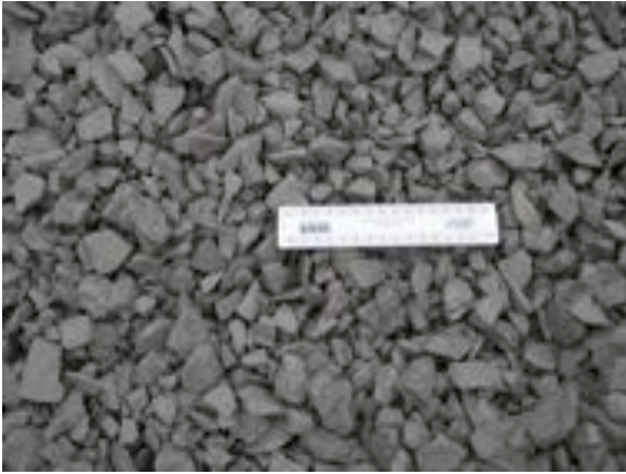
Permeable subbase (4/20 material)
